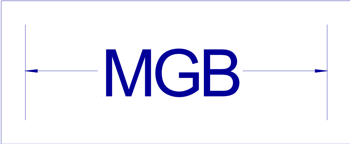
Figure 4-3 Designation of MGB when it is Part of a Power Plant's Battery Return Bus
